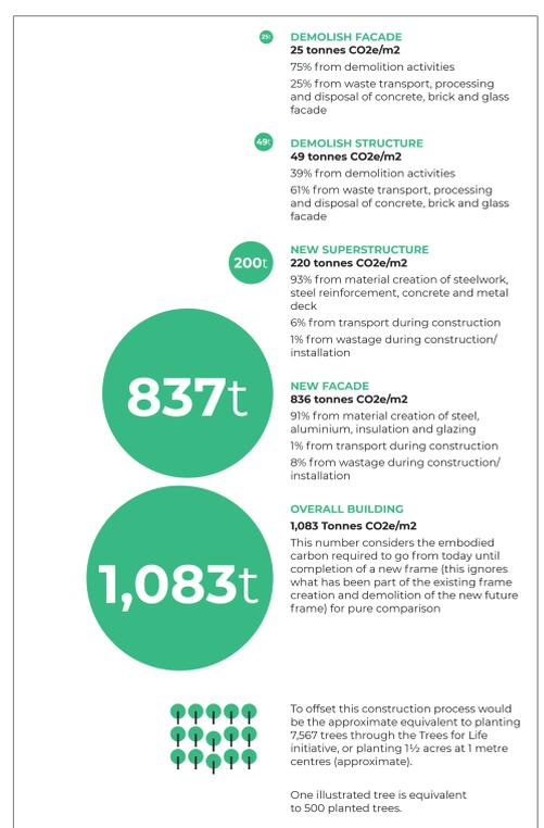
Diagrams comparing the embodied carbon of the two different design options.
